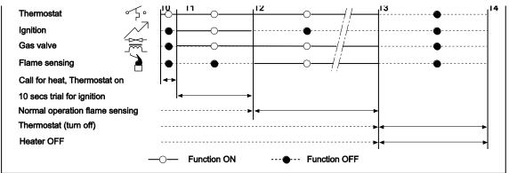
If the flame is not sensed during sequence T2 then the burner will automatically begin re-ignition sequence T1. The ignition sequence will be repeated three times with a 15 second inter-purge. If the flame is not reestablished the heater will go to lockout.
